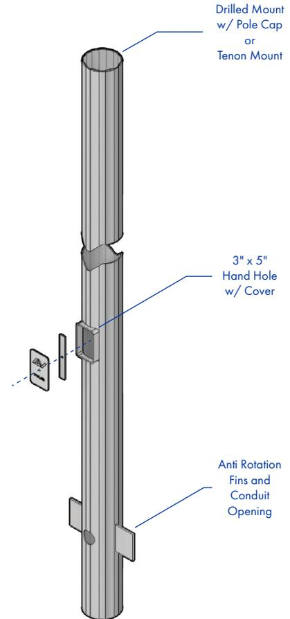
**SHAFT:** One-piece extruded 6063 aluminum alloy tube heat treated to a T6 temper.
