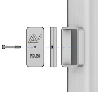
**HAND HOLE:** Reinforced 3" x 5" hand hole is located 18" above grade. Cover and attachment hardware provided.
